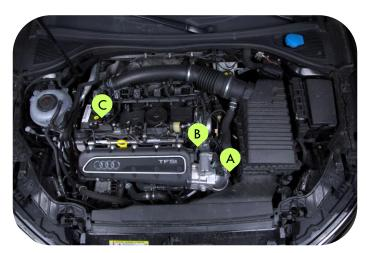
Harness Section A – Turbo Boost Pressure Sensor – Route section A down under the airbox and towards the front of the engine, Disconnect the turbo boost pressure sensor connecter and wire in series the PCM wiring harness section labelled A. See figure 3a for assistance.
